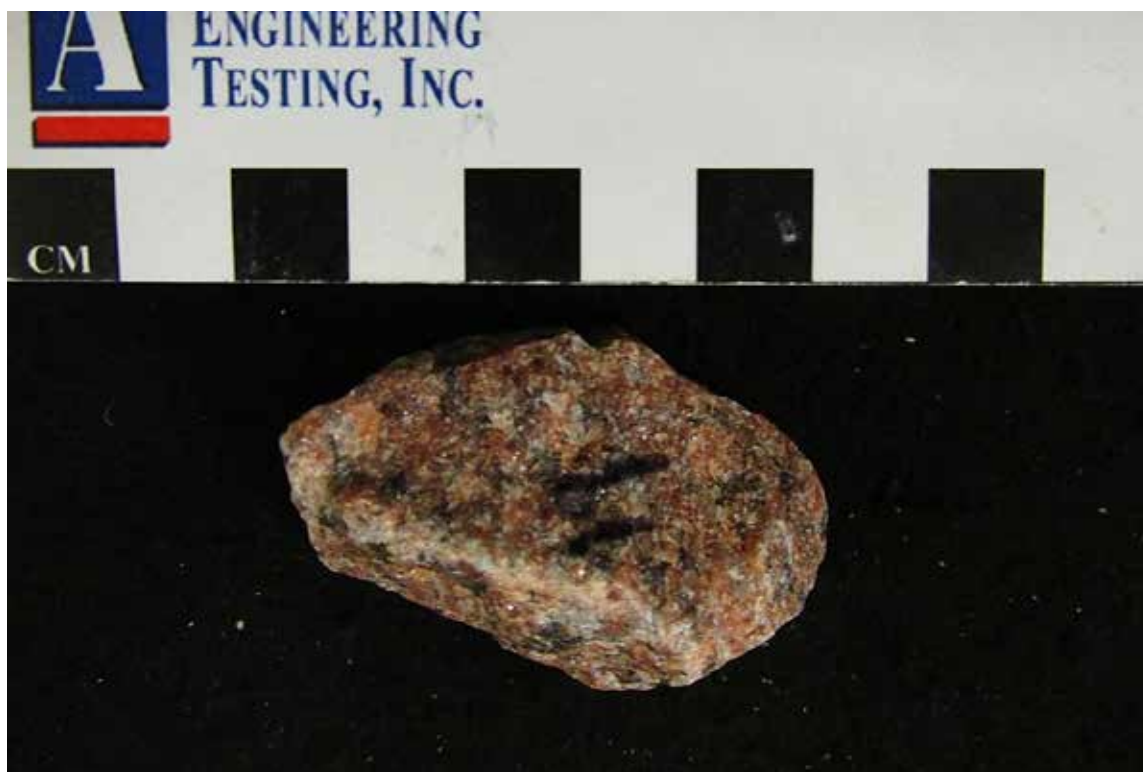
SAMPLE ID: #19 Sunset Pink Granite DESCRIPTION: View of the stone selected for hardness testing.
