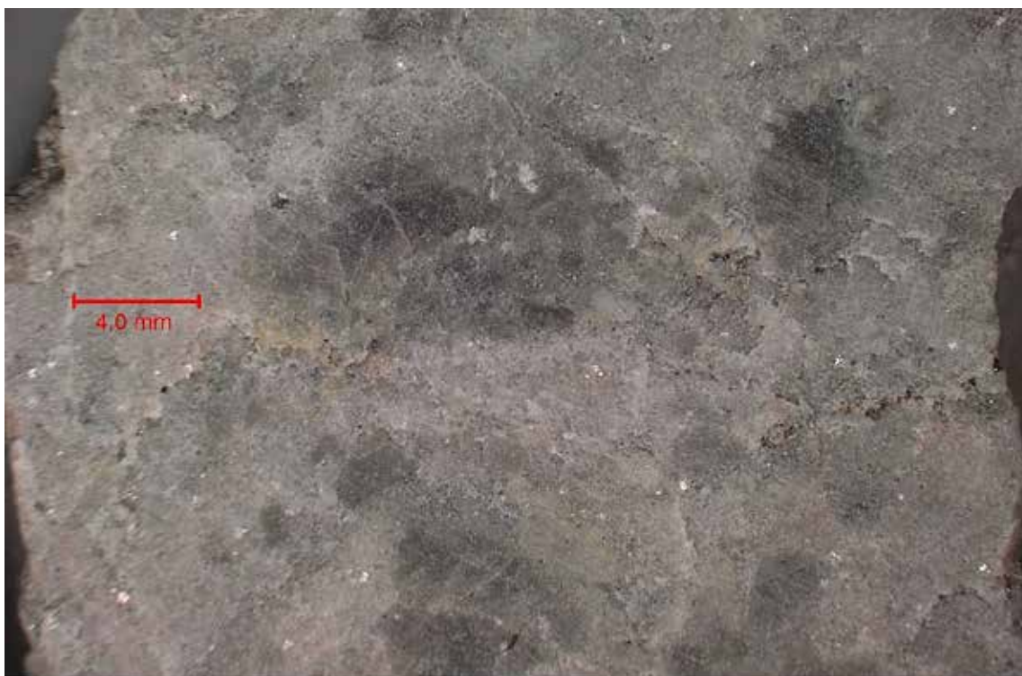
SAMPLE ID: #10 Misty Grey Marble MAG: 5x DESCRIPTION: View of the lapped cross section of the stone.
