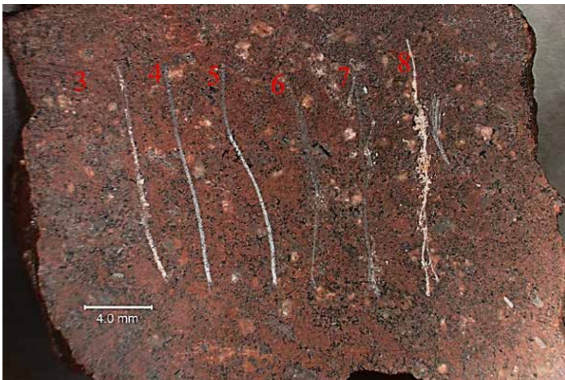
SAMPLE ID: Sample #3-Wineberry 3/8x1/8 MAG: 5x DESCRIPTION: View of the lapped cross section of the stone after Mohs hardness testing. Note that hardness picks 3, 4, 5, and 6 did not scratch, hardness pick 7 scratched a few minerals, and hardness pick 8 scratched all minerals. The general Mohs hardness would be approximately 7.
