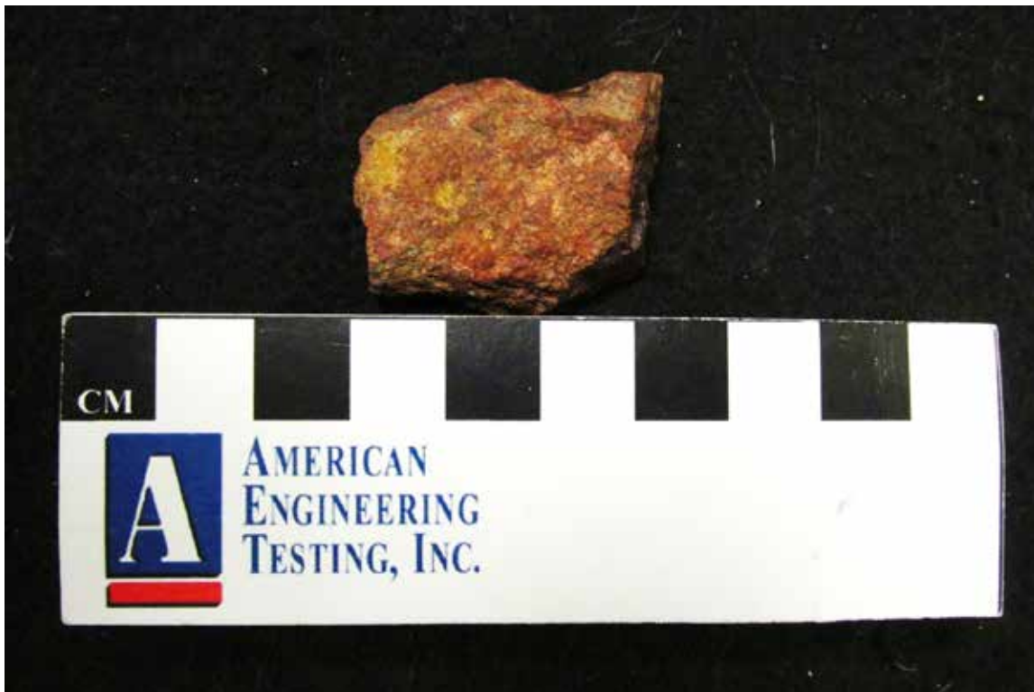
SAMPLE ID: Sample #3-Wineberry 3/8x1/8 DESCRIPTION: View of the stone selected for hardness testing.
