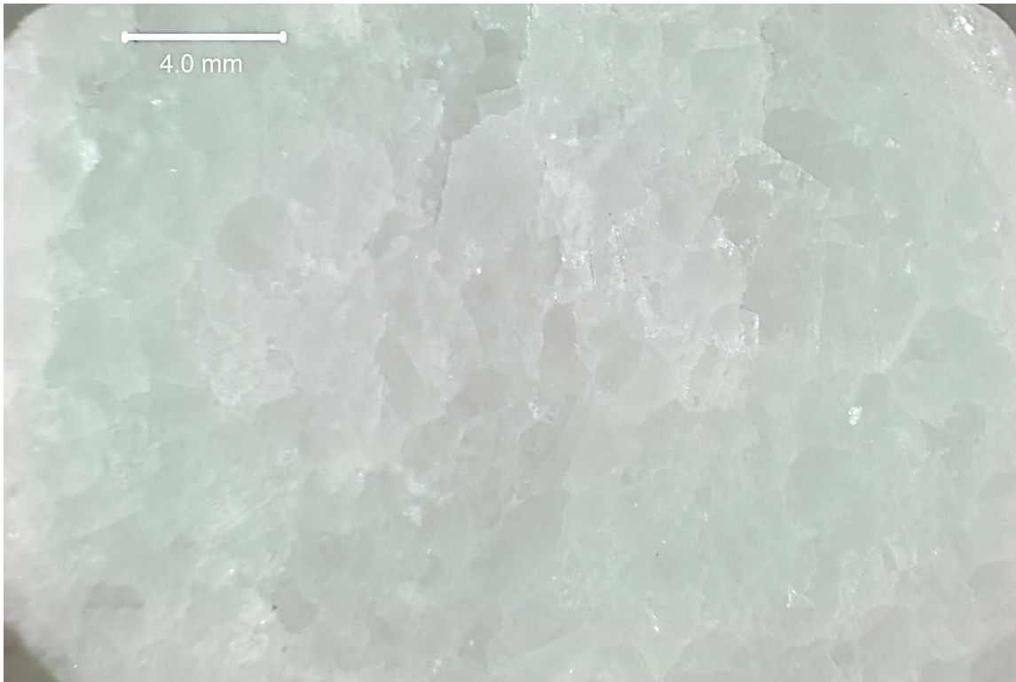
SAMPLE ID: 3/8" x 1/8" Super White MAG: 5x DESCRIPTION: View of the lapped cross section of the rock.
