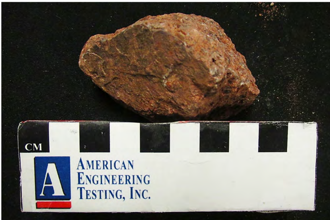
SAMPLE ID: Red Cedar Granite DESCRIPTION: View of the stone selected for hardness testing.
