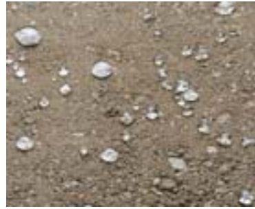
Water shedding off of compacted surface.
