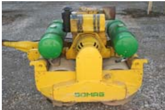
Compaction of wet granular base
